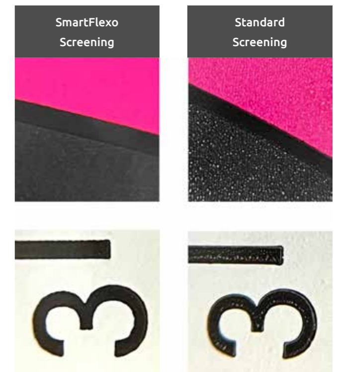
↑ Xitron's SmartFlexo optimises plates and press response by selecting the AM to FM transition point. The technology eliminates trailing edge voids and maintains dots in hard-to-hold highlight areas with multiple SmartDot choices.
